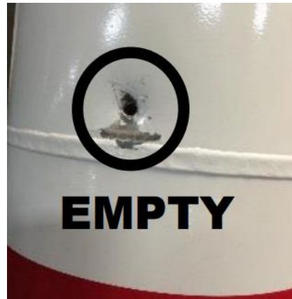
Empty flammable refrigerant cylinder
