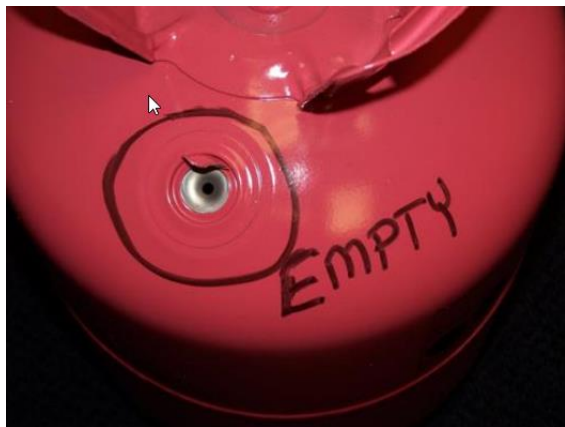
Empty non-flammable refrigerant cylinder
